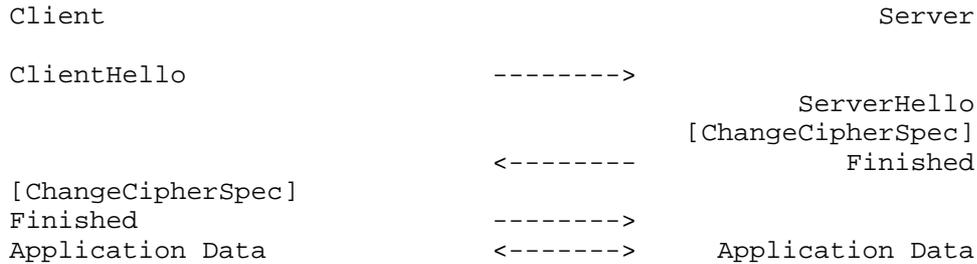
Fig. 2 - Message flow for an abbreviated handshake
