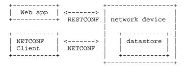
The following figure shows the system components if a RESTCONF server is implemented in a device that does not have a NETCONF server:
