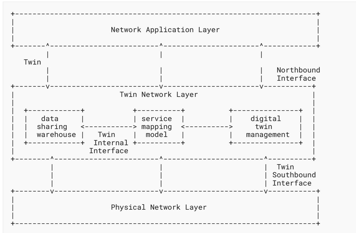
Figure 1: Schematic Representation of DTN Interface
